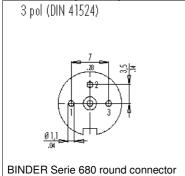
PIN 1: RS232 RX PIN 2: RS232 TX PIN 3: RS232 GND
